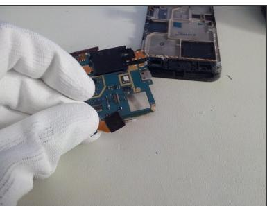
Use the removal tool to unclip the camera module from the Logic board.
