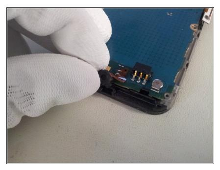
• Lift the microphone from the logic board.
