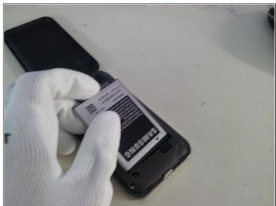
Remove the battery cover and the battery
