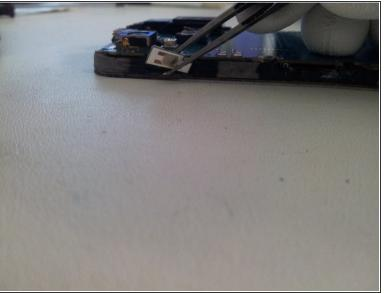
• Use a flat tweezer for take off the flexible on/off button from the frame.
