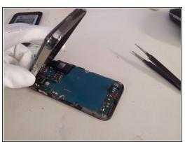
Lift gently the back cover from the screen assembly from the bottom.
