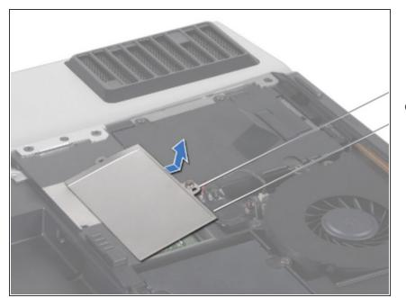
Slide the memory-module door to release the tabs and lift the memorymodule door out of the computer base.
