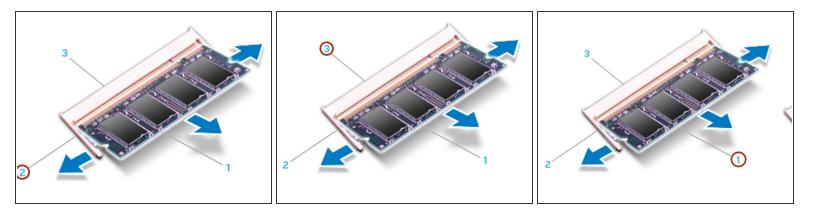
CAUTION: If you need to remove memory modules from both connectors, remove the memory module in the upper connector before you remove the module in the lower connector.
