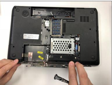
Remove service hatch by sliding away from the computer and lifting up.
