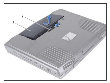
Align the tabs on the **NEW** battery with the slots on the battery bay and snap the battery into place.
