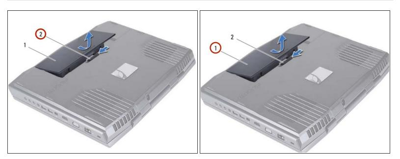
Slide the battery latch to the unlock position as shown. The battery pack pops up.
