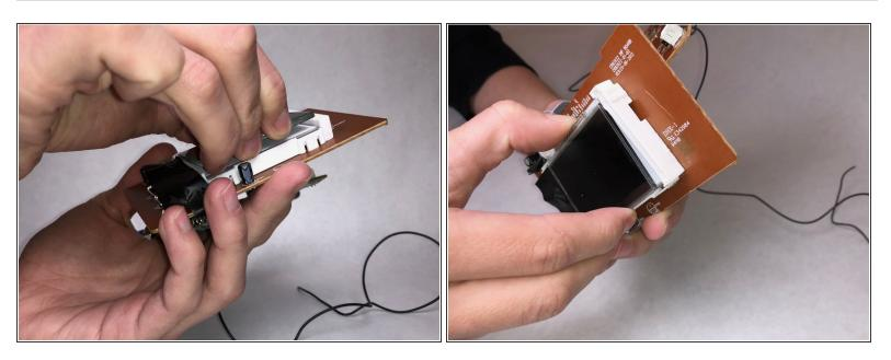
Lift the screen upward, taking care not to allow the films below it to fall out.
