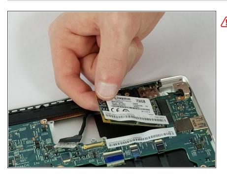
Remove the hard drive by pulling it away horizontally from its connection.
