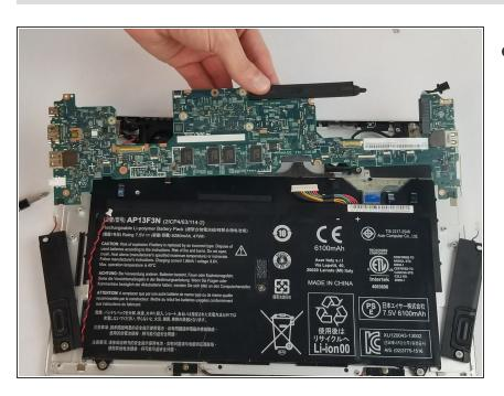
Lift up on the motherboard to pull it out of the casing.
