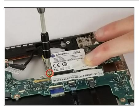
Remove the marked 2mm screw with a Phillips #01 screwdriver.
