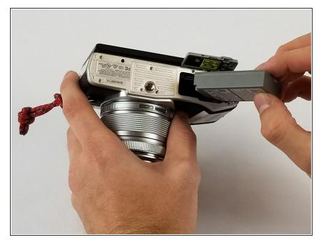
• You can now remove the battery from the body of the camera and begin reassembly with your new battery.
