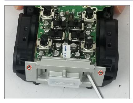
Turn device 180 degrees to unscrew two (PH #1), 8mm screws from the mic connector.
