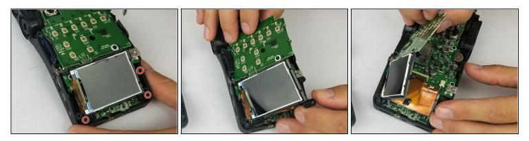
• Unscrew three (PH #1), 7mm screws from the button board near the display and gently flip over.
