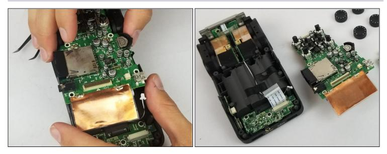
• Gently lift off motherboard from the base of the device.
