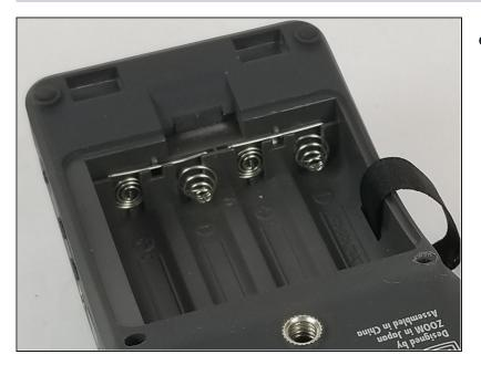
• If batteries are present, remove them in order to reveal the terminals at the bottom of the device.
