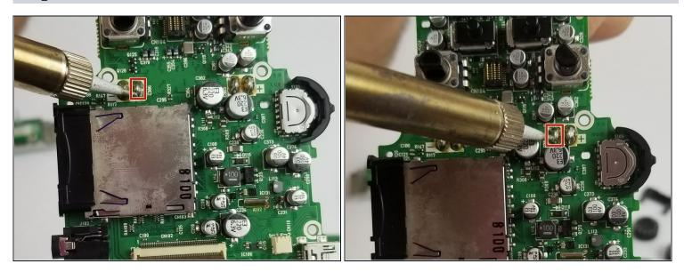
• Taking care not to damage other components on the motherboard, use a soldering iron to undo the soldering that holds the terminals to the motherboard.
