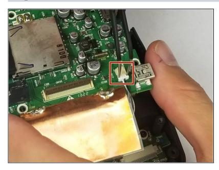
Disconnect wire from motherboard using <u>tweezers</u>.
