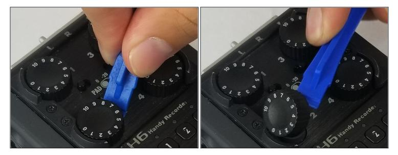
• Place device face up and remove the four knobs using the flat end of the plastic opening tool.
