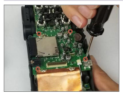
• Unscrew four (PH #1), 8mm screws from the motherboard.
