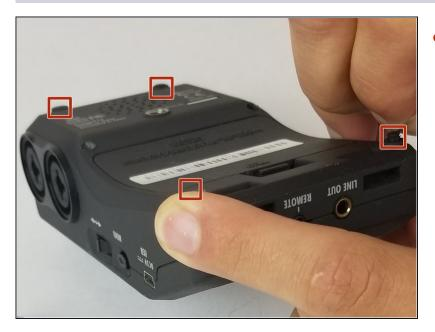
Remove four rubber feet using fingernails to access the four screws underneath.
