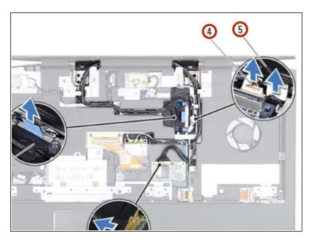
Disconnect the camera cable and infrared cable from the respective system board connectors.
