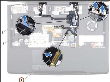
Route the display cable, camera cable, infrared cable, wirelessHD card cable, and Mini-Card antenna cables through the routing guides on the palm rest assembly.
