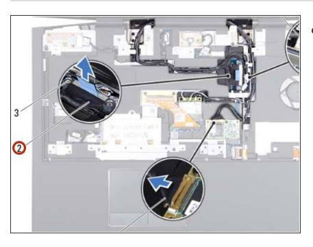
Using the pull-tab, pull the display cable to disconnect the display cable from the connector on the system board.
