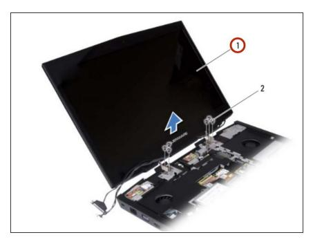
Lift the display assembly off the computer.
