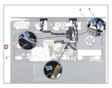
Tighten the captive screws that secure the display cable to the system board.
