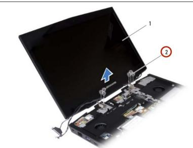
Place the NEW display assembly in position and replace the screws that secure the display assembly to the computer base.
