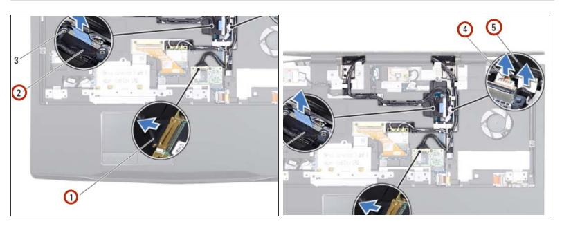
Note the routing of the display cable, camera cable, infrared cable, wirelessHD card cable, Mini-Card antenna cables and remove the cables from the routing guides on the palm rest assembly.
