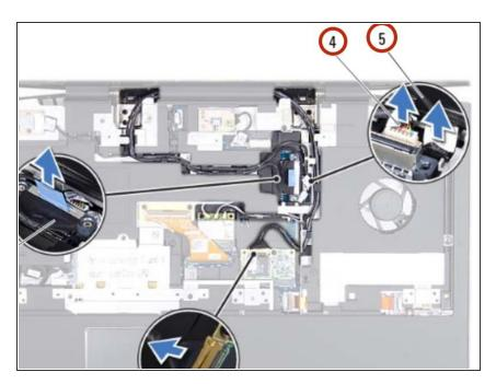
Connect the camera cable and infrared cable to the respective system board connectors.
