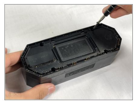
Remove the four 13.7mm Phillips #1 screws located underneath the rubber stoppers.
