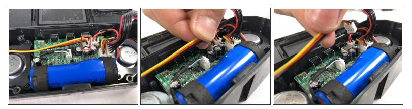
To remove the speaker, gently pull out the its wire harness.
