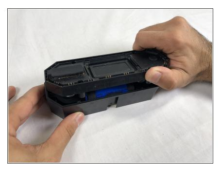
• Pull the case apart to access the interior components.
