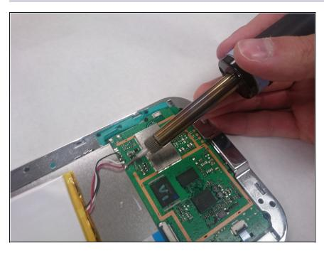
• <u>Desolder</u> the battery wires from the circuit board.
