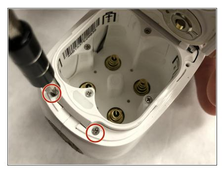
Open the battery cover and remove the 2 (3.5mm") screws from under the cover.
