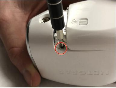
• Slide the unlocked battery cover forward to remove 2 (3.5mm) screws, that are behind the cover.
