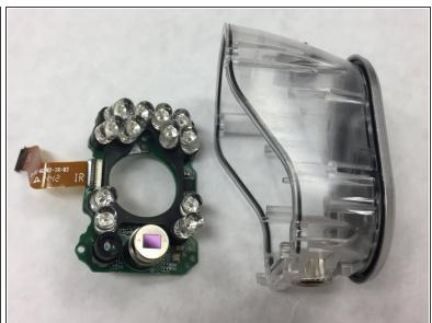
Use the plastic opening tool to slowly pry the board away from the front housing.
