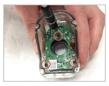
Remove 3 (.150") screws from the sync board using the JIS00 screwdriver.
