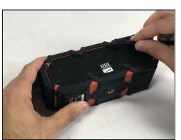
Use the spudger to remove the eight black pins from the front and back of the wire screens.
