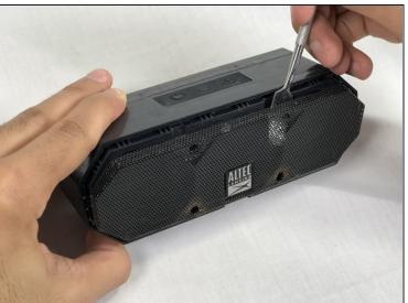
Pry off the wire mesh on both sides using a metal spudger.
