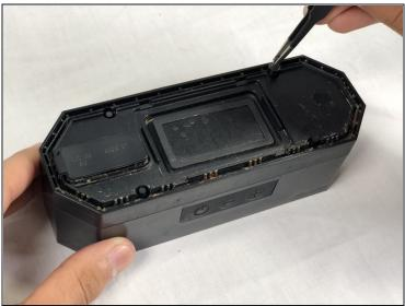
• Using <u>tweezers</u>, remove the four rubber stoppers in each corner of the rear panel.
