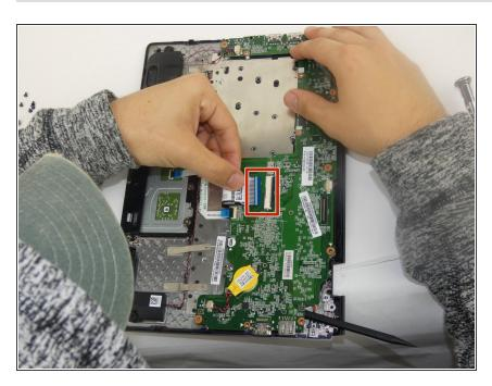
Lift up black flap on the ZIF connector and pull the ribbon cable out.
