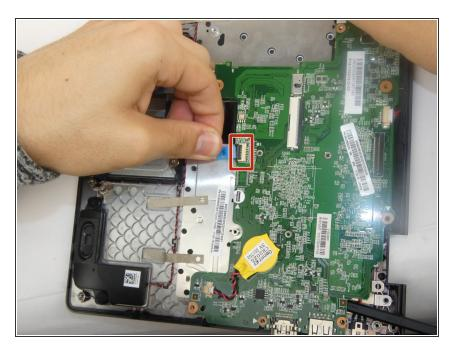
Lift up on the black tab on the ZIF connector and pull the ribbon cable out.
