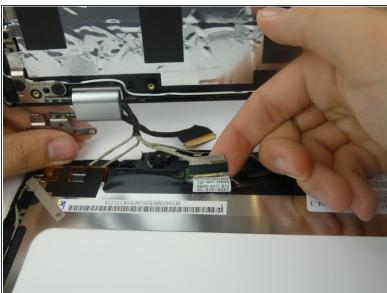
Peel off tape and remove the cable.
