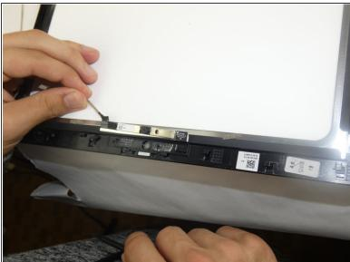
Peel tape and remove cable underneath.
