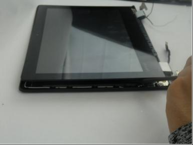
• Use the black nylon spudger to lift and separate the screen from the plastic back cover.
