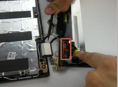
Remove the connector chip.
