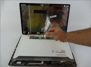
• Remove the tape completely from the back panel.
