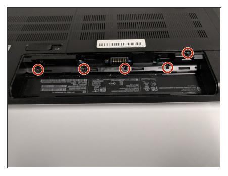
Remove the five marked screws found under the battery using a philips head screwdriver.
