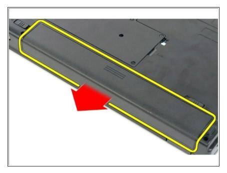
Slide the battery toward the back of the computer to remove.
