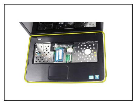
Pry up the palm rest using a plastic scribe to release all the snaps on the bottom, left, and right sides of the palm rest. Once all the snaps have been released, lift up the palm rest from the computer and remove.
