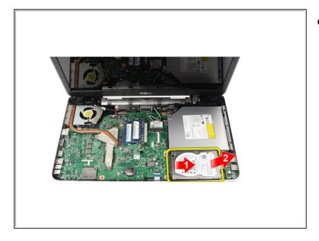
Remove the screws that secure the hard drive bracket and detach it from the hard drive.
