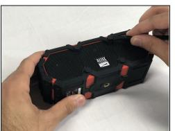
Use the spudger to remove the eight black pins from the front and back of the wire screens.
