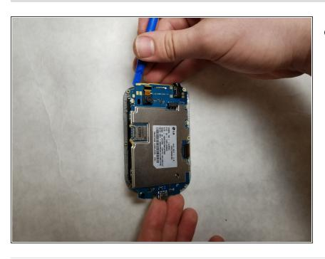
Pry the screen from the internal circuit board with a plastic opening tool and remove it.
