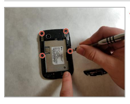
Remove the four 4 mm screws using a JIS screwdriver with a J000 head from the top part of the internal casing.
