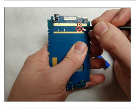
Detach the camera completely by using the spudger tool to poke through the camera attachment holes.
