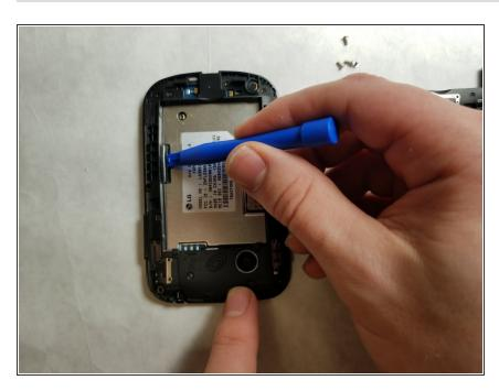
Pry open the top part of the internal casing with the plastic opening tool and remove it.
