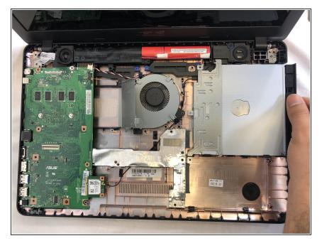
Remove the disc drive by sliding it towards the right and removing it from the laptop case
