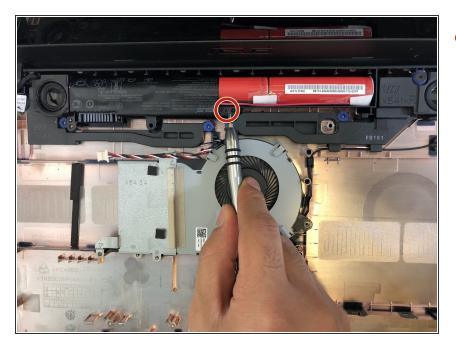
Remove the 6mm Phillips #0 screw from the battery bracket.
