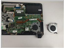
Use long nose tweezers to remove connector. Fan will lift out.
