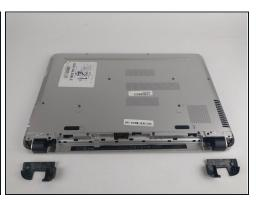
• With the battery removed, remove both black plastic covers with a plastic opening tool. Unscrew both 7.5 mm screws from the tabs, using a PH1 screw driver. Using a plastic opening tool, pry off both covers.
