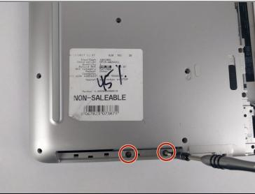
• With the CD drive removed, unscrew the two 2mm silver screws with a PH00.
