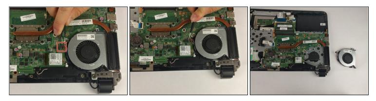
Use long nose <u>tweezers</u> to remove connector. Fan will lift out.
