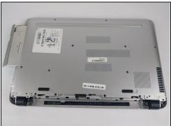
• Remove all 16 of the 3.5 mm screws with a PH1 screwdriver and pry/slide the CD drive out of laptop.
