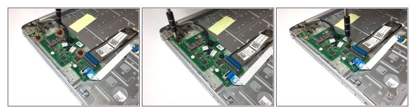
Remove the 3, 2.5 mm screws on the circuit board.
