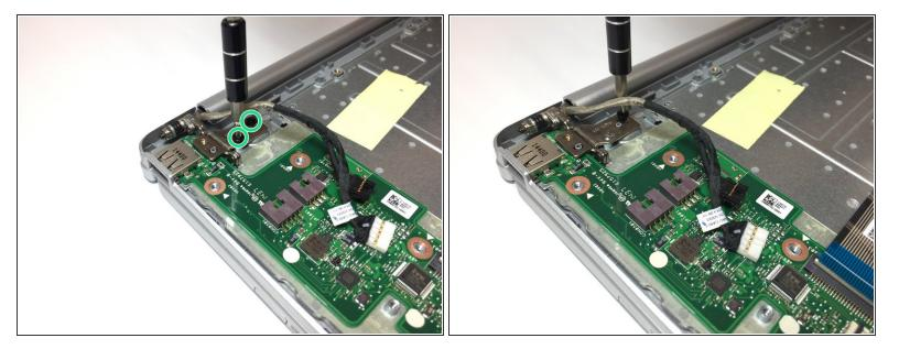
Remove the 2, 4.25 mm screws on the security tab.
