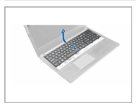
Slide and lift the keyboard to access the keyboard connector cable under the keyboard [1,2].
