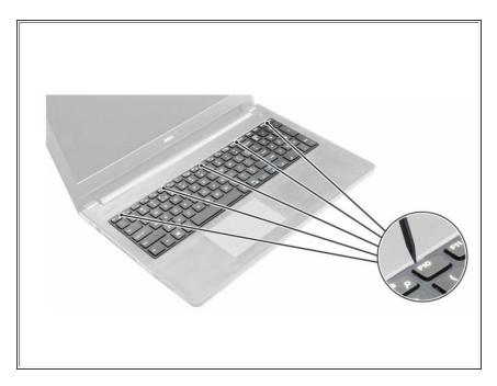
Release the keyboard by prying on the keyboard release tabs by using a scribe.
