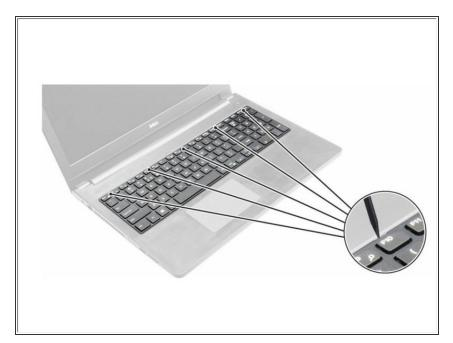
Release the keyboard by prying on the keyboard release tabs by using a scribe.
