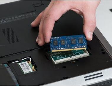
With the holding clips unfastened, lift the RAM from its socket.
