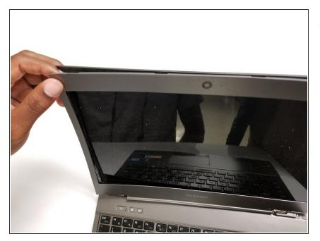
Detach the frame from the housing clamps around the perimeter of the screen.
