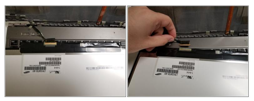
• Disconnect the <u>display cable connector</u> from the screen.
