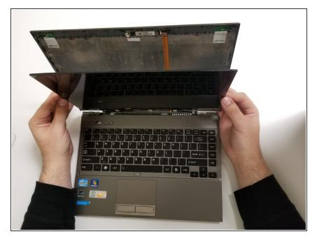
Remove the screen from its fasteners around the perimeter of the upper half.
