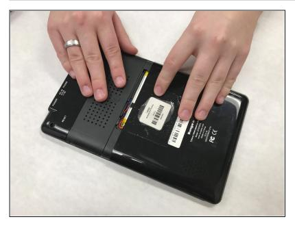
• Press firmly on lower portion of the back cover and slide the cover towards the bottom to remove cover.
