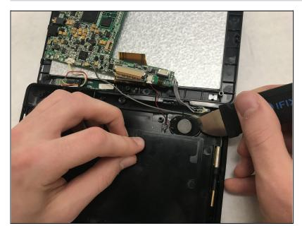
Pry the speaker out of retainer clip with iFixit pry tool.
