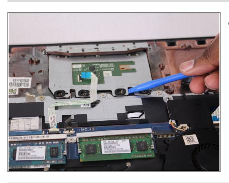
Use the plastic opening tool to lift the touchpad up and pull out to remove.
