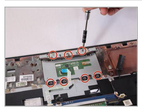
Remove the seven 3mm Phillips #00 screws from the trackpad.
