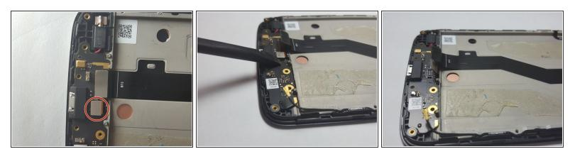
Use the <u>Spudger to lift up and detach the Fingerprint Scanner Flux Cable</u> from the <u>Cable Port</u>.
