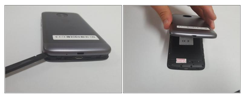
• Insert the spudger into the notch on the corner of the phone and lift up to remove the back case.
