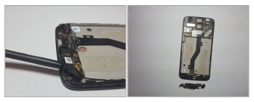
• Use the <u>Spudger</u> to lift up and remove the <u>Charging Port</u> from the phone. The black box connected to the charging port will lift up with it. Remove the whole piece.
