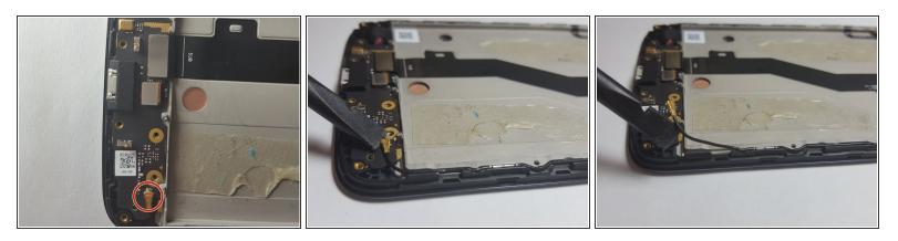
Use the <u>Spudger</u> to lift up and remove the <u>Signal Flux Cable</u>, circled in picture, from the <u>Cable</u> <u>Port</u>. The <u>Signal Flux Cable</u> should still be connected to the side of the phone, but detached from the charging port.
