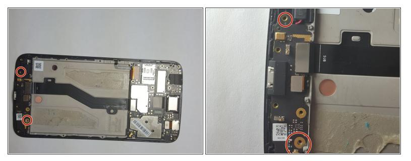
• Use the <u>T4 Torx Screwdriver</u> to remove the <u>two 3.2 mm screws</u> circled.
