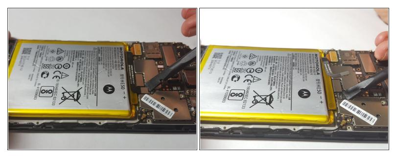
After removing the back panel, use the spudger to lift and detach the <u>Battery Flux Cable</u> from the <u>Motherboard</u>.
