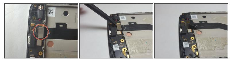
Use the <u>Spudger</u> to lift up and detach the <u>Main Flex Cable</u> from the <u>Cable Port</u>.
