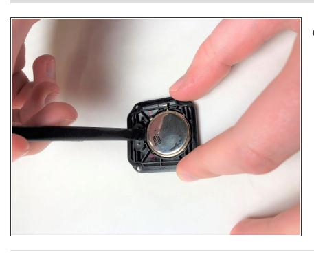
Pry the old battery out using a plastic spudger.
