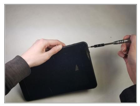
Using the PH00 screwdriver, remove the two 4mm screws located on both the left and right sides of the charging port on the bottom of the tablet.
