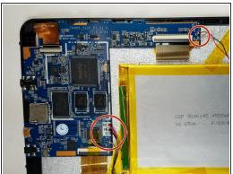
• Using a soldering iron, desolder the points circled on the picture until the solder have liquefied enough to be able to remove the wires from the circuit board.
