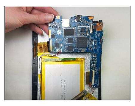
Gently lift the circuit board from the housing. You have now successfully removed the circuit board. Now, you can insert the new board to the tablet.
