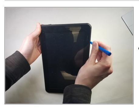
Using the plastic opening tool, insert it into the crease where the glass screen meets the housing of the rest of the tablet. Once inserted, keep inserted and run along the edges to separate the plastic clips from each other to dislodge the back plastic away from the glass and internal components.
