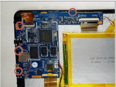
Using the PH00 screwdriver, unscrew the four 4.4 mm screws that are anchoring the circuit board down to the rest of the tablet.
