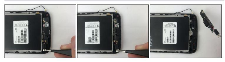
• Insert the tweezers under the vibrator and gently lift up the whole part.
