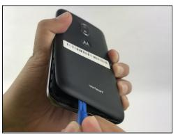
• Open case with a plastic opening tool that has the same size as the divot located at the bottom left of the phone. If you don't have an opening tool, use your finger nails.
