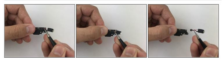
• Pop up on the vibrator's connector to separate it from the charging port.
