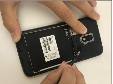
• Remove the small silicon cover at the bottom right of the camera using <u>tweezers</u>.
