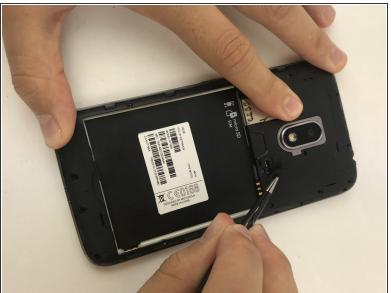
Remove the small silicon cover at the bottom right of the camera using tweezers.
