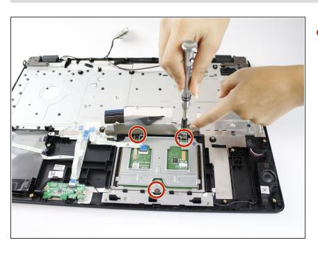
Remove the three 6mm Phillips #0 screws from touchpad.
