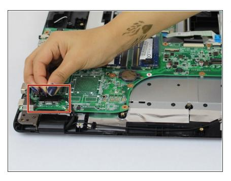
Disconnect the display cable from the motherboard.
