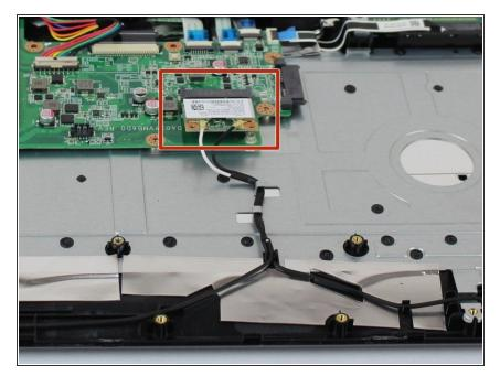
Remove the Wi-Fi card by pulling it from the motherboard socket.
