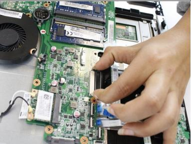
Use a spudger to flip up the retaining flap on the black ribbon cable <u>ZIF</u> socket.
