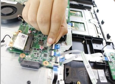
Use a spudger to flip up the retaining flaps on the ribbon cable <u>ZIF</u> sockets.
