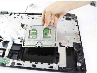
Lift the touchpad up by the side closest to the middle of the laptop and pull up towards you to remove.
