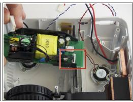
Slide out the power source and disconnect its cables from the power jack and the light.
