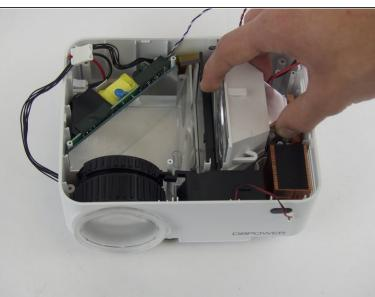
Remove the two (3 mm) screws connecting the bracket down and pull out the reflector, using a J0 Philips Head Screwdriver.
