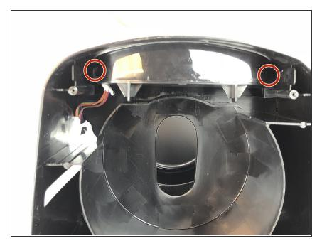
Remove the two 1.3mm Phillips #0 screws from the display.
