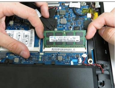
Place your fingernail or a pry tool in between the metal retention bars and the RAM unit.
