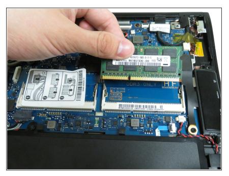
Pull up on the RAM unit at a 45 degree angle to release it from the retention bars.
