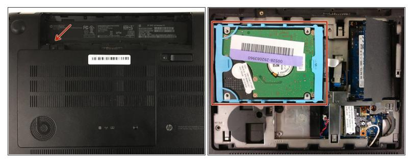
• Remove the small panel on the back by prying it off. This should reveal the hard drive.
