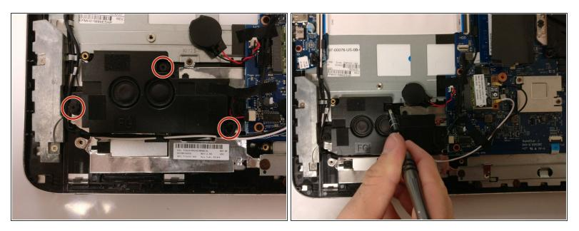
Use a screwdriver to unscrew the three screws on the speaker.
