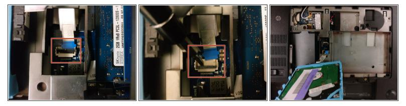
(i) The hard drive is connected to the motherboard via this blue-tabbed cable, highlighted in red.
