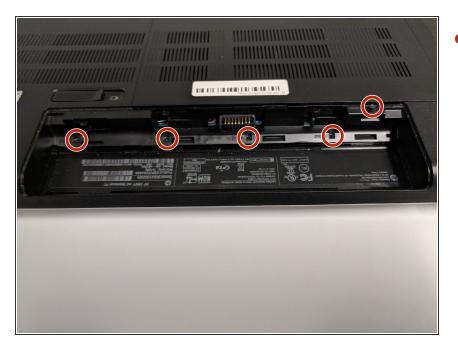
Remove the five marked screws found under the battery using a philips head screwdriver.
