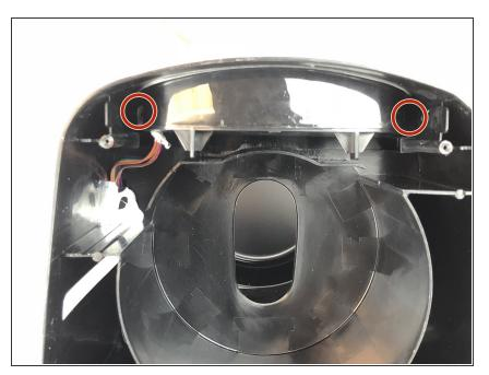
• Remove the two 1.3mm screws from the display.
