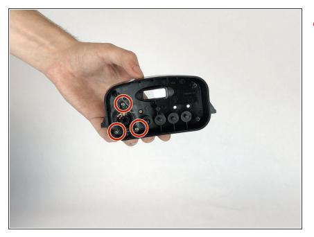
Remove the three 1mm Phillips #0 screws from the knob.
