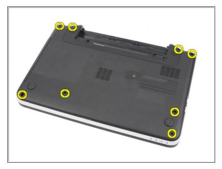
Remove the screws that secure the bottom base.
