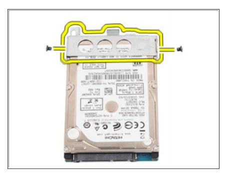
Remove the screws that secure the hard drive bracket and detach it from the hard drive.
