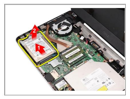
Slide the hard drive and lift it out of the computer.
