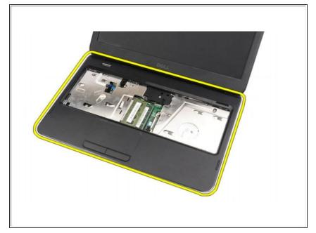
Pry up the palm rest using a plastic scribe to release all the snaps on the bottom, left, and right sides of the palm rest. Once all the snaps have been released, lift up the palm rest from the computer and remove.
