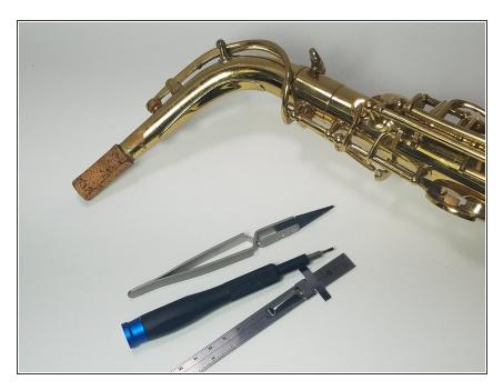
Before any actions are taken, you should check the simplest possible fixes. Remove the neck and tap the back of the arm. If it moves freely and does not stick, you may skip to step 4.
