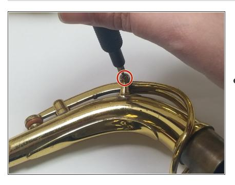
when tapped. The least likely issue to impact the arm's performance is an overly tightened screw that holds the arm and allows it to pivot. If this screw is too tight, it causes the frame the arm sits in to constrict and prevent movement.
