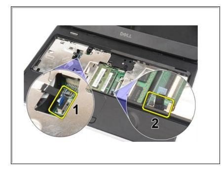
Flip the computer around and disconnect the power board cable (1) and the touchpad cable (2).
