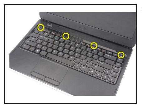
• Pry up to release the top four snaps securing the keyboard to the computer.
