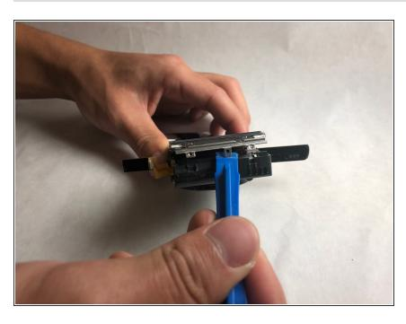
Working on the left side of the screen, pry the metal panel off from the motherboard housing using a plastic opening tool.
