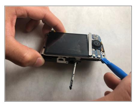
Pry back the panel to the right of the screen using a plastic opening tool.
