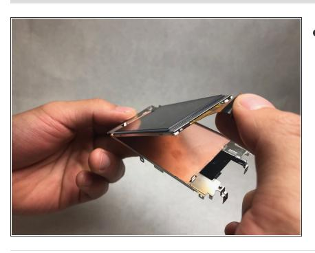
Lift the LCD screen from it's metal housing.
