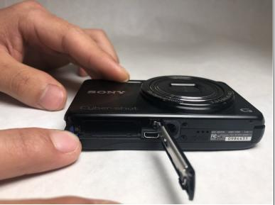
Pull down on the blue tab to release the battery.
