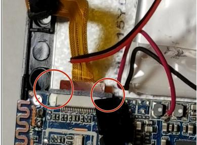
Use the plastic spudger to pry the tabs open on the digitizer ribbon sockets.
