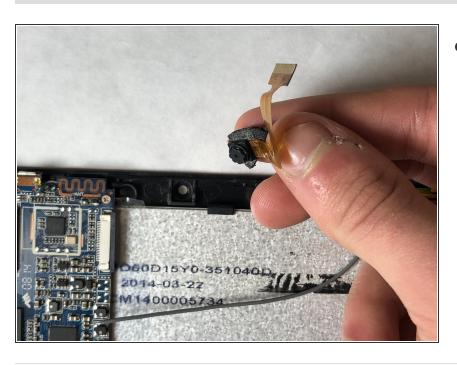
Pull the camera out of the device.
