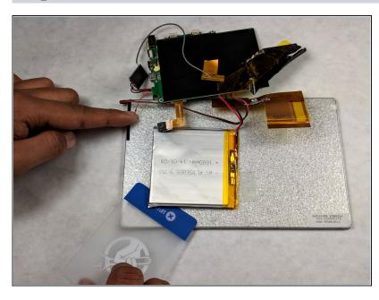
• Using a <u>plastic card</u>, gently remove the adhesive that holds the battery in place and separate the battery from the LCD panel.
