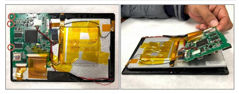
• Remove the three 4 mm JIS #0 screws to release the PCB board.
