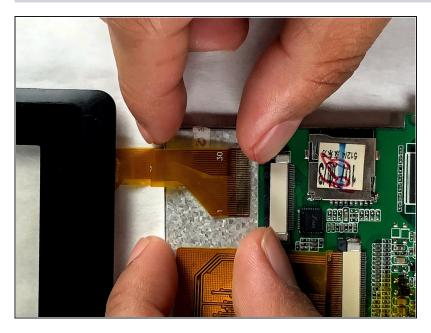
Using both hands, gently release the ribbon cable to the capacitive touch screen overlay from the PCB board by pushing both gray tabs outwards.
