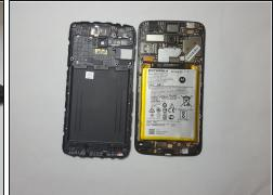
Lift up and remove the back panel.
