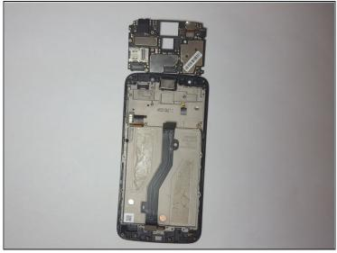
• Use the <u>Spudger</u> to lift up and remove the <u>Motherboard</u> from the phone.
