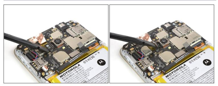
• Use the flat end of a spudger to pry up and disconnect the rear camera flex cable.
