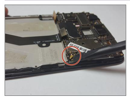
Use the <u>Plastic Spudger</u> to lift up and detach the <u>Signal Flex</u> <u>Cable</u> from the <u>Motherboard</u>. The <u>Signal Flex Cable</u> should still be attached to the body of the phone.
