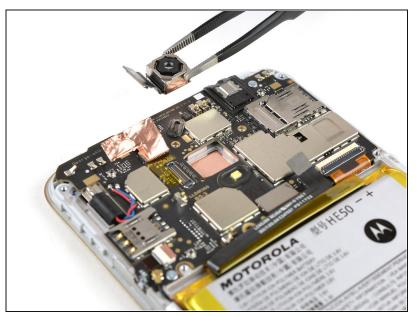
• Carefully remove the rear camera with a pair of tweezers.
