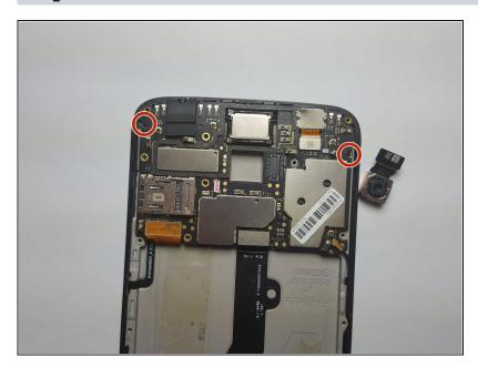
• Use the <u>T4 Torx Screwdriver</u> to remove the <u>2 3.2 mm screws</u> circled in the image.
